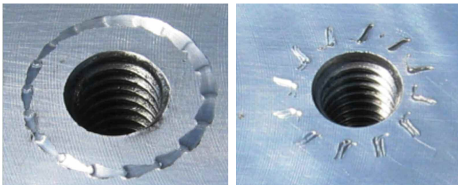
“Raptor tracks” vs. “lock washer scratch” of equally torqued fastener
